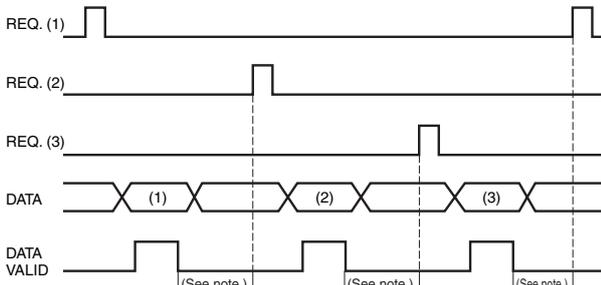
**Note:** Leave 20 ms min. between DATA VALID turning OFF and the REQUEST signal.
