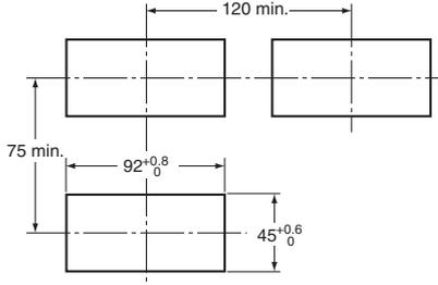
Mounting Recommended Panel Thickness 1 to 8 mm. Mount the product horizontally.
