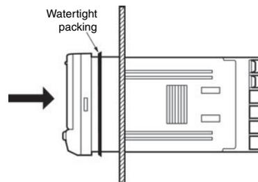
3. Insert the adapter into the grooves on the left and right sides of the rear case and push until it reaches the panel and is fixed in place.
