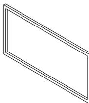
(Depending on the operating environment deterioration, contraction, or hardening of the rubber packing may occur and so, in order to ensure the level of waterproofing specified in NEMA4, periodic replacement is recommended.)
