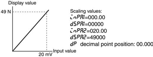
**Note:** “2 mV/V” indicates a load cell output of 2 mV for 1 V applied voltage for the rated load (when using a load of 1 N). When the applied voltage is 10 V, the load cell output is 20 mV (2 mV × 10). The precision can be increased by entering the A1 and A2 input values by teaching, and then scaling the results.
