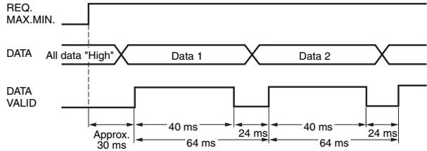
Measurement data is output every 64 ms while the REQUEST signal remains ON.
