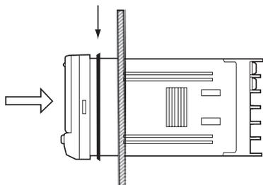
3. Fit the adaptor into the grooves on the left and right sides of the rear case, then push it until it contacts the panel to secure the K3MA-J.
