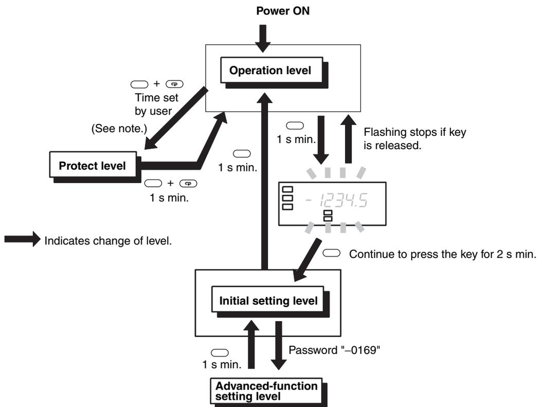
**Note:** The move-to-protect-level time can be set in the advanced-function setting level.
