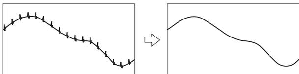
This is useful for ignoring rapid fluctuations, e.g., eliminating spike noise.
