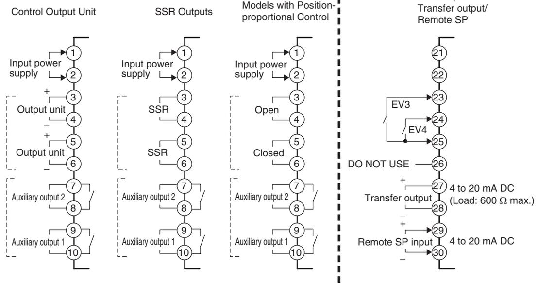
**Note:** Wire all voltage input terminals correctly. The Controller may fail if voltage input terminals are wired incorrectly.
